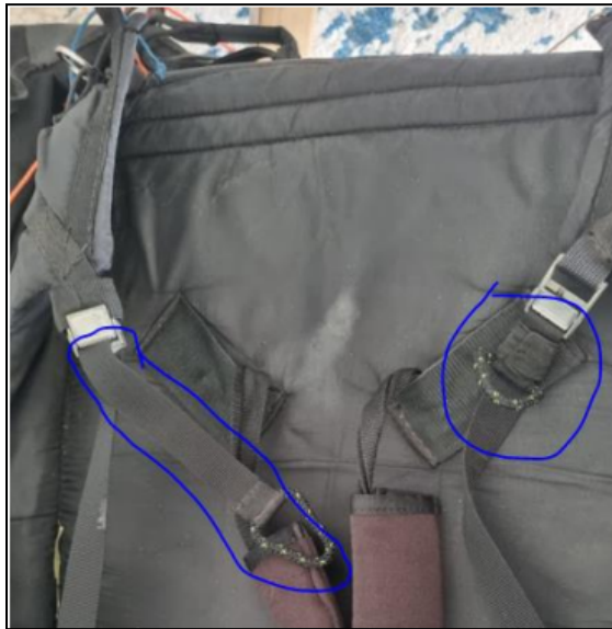
Figure 22: Harness setup showing leg straps asymmetry
